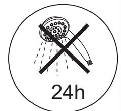
Warning: Don't use the shower enclosure until after at least 24 hours, so that the silica gel can be totally dry.
